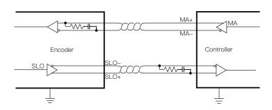
It is a four-wire interface, include the differential lines of MA and SLO. And the terminal resistors of the MA lines have been integrated into the encoder. The users only need to configure terminal resistors or choose other impedance matching schemes for SLO lines.
