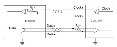
It is a four-wire interface, include the differential lines of Clock and Data. And the terminal resistors of the Clock lines have been integrated into the encoder. The users only need to configure terminal resistors or choose other impedance matching schemes for Data lines.
