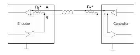
It is a differential two-wire interface, both wires need to be terminated with parallel termination resistors. The terminal resistors have been integrated into the encoder. The users only need to configure terminal resistors or choose other impedance matching schemes for the differential wires of the controller side.
