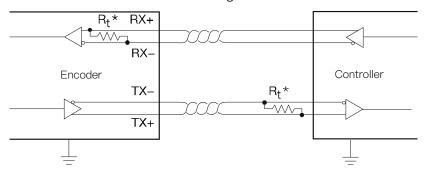
It is a four-wire interface, include the differential lines of TX and RX. And the terminal resistors of the encoder RX lines have been integrated into the encoder. The users only need to configure terminal resistors or choose other impedance matching schemes for TX lines.
